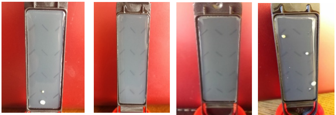
Hygicult Contact Slides showing the Cfu count on the handles Post-installation
