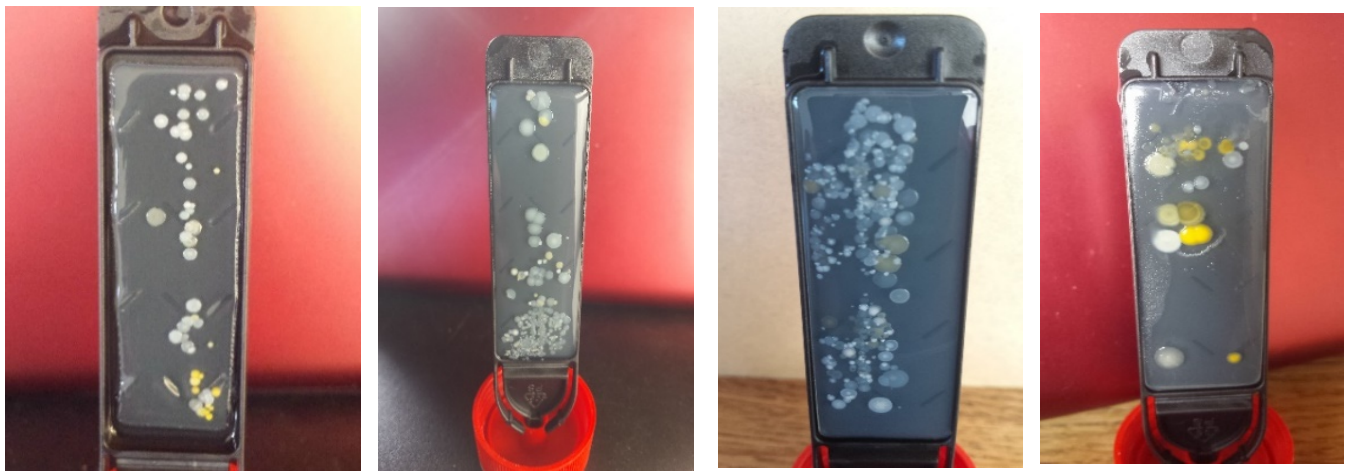
Hygicult Contact slides showing the Cfu count on the handles Pre-installation .
